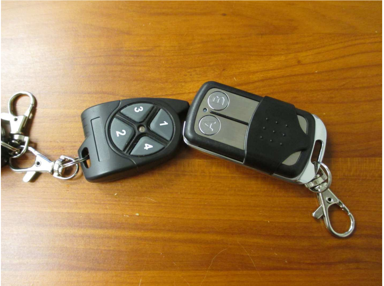
Picture shown the position of the transmitters when using transmitter PL-CRC-I11 to copy the code from transmitter PL-RC-C1
