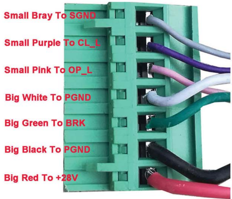
Straight 7-Pin Connector Wiring Diagram
