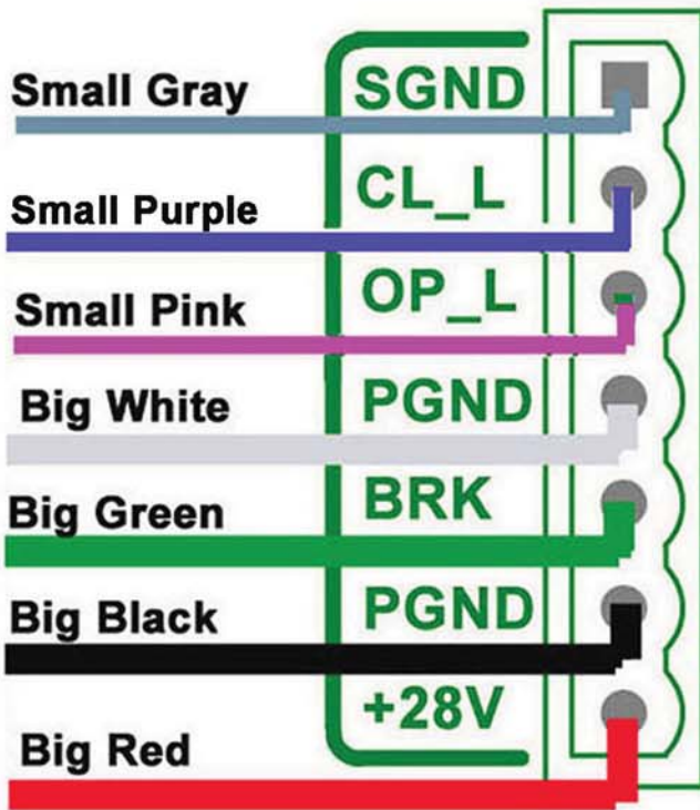
Straight 7-Pin Connector Wiring Diagram
