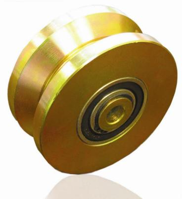
4" Platinum VGW-3000 steel V-Groove wheel holds gates up to 3000lbs per wheel. It is designed for high traffic that use for commercial and residential sliding gate track application. VGW-3000 is designed to be maintenance free. VGW-3000 is made by machining from solid cold rolled steel. It comes with sealed bearings.
