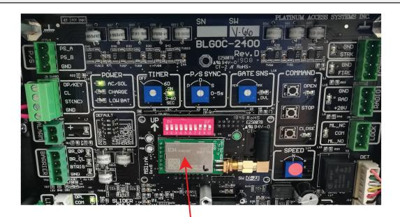
Plug in the MSLink module to the BLGOC-2400 main board.
