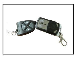
Picture shown the position of the transmitters when using transmitter PL-CRC-I11 to copy the code from transmitter PL-RC-C1
